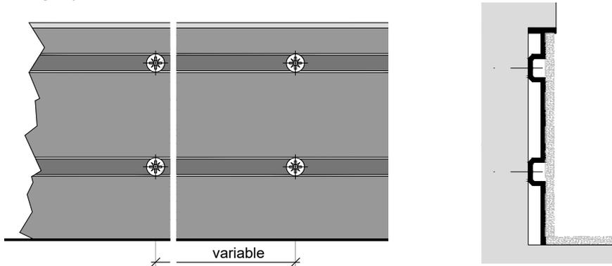
In those cases when 2-parted profiles are mounted, the basic profile must be aligned precise! Only then a mounting of the cover profile is possible.
